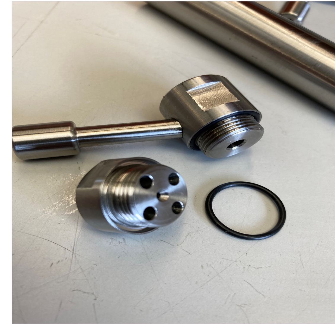
Atomiser ends waiting to be assembled
