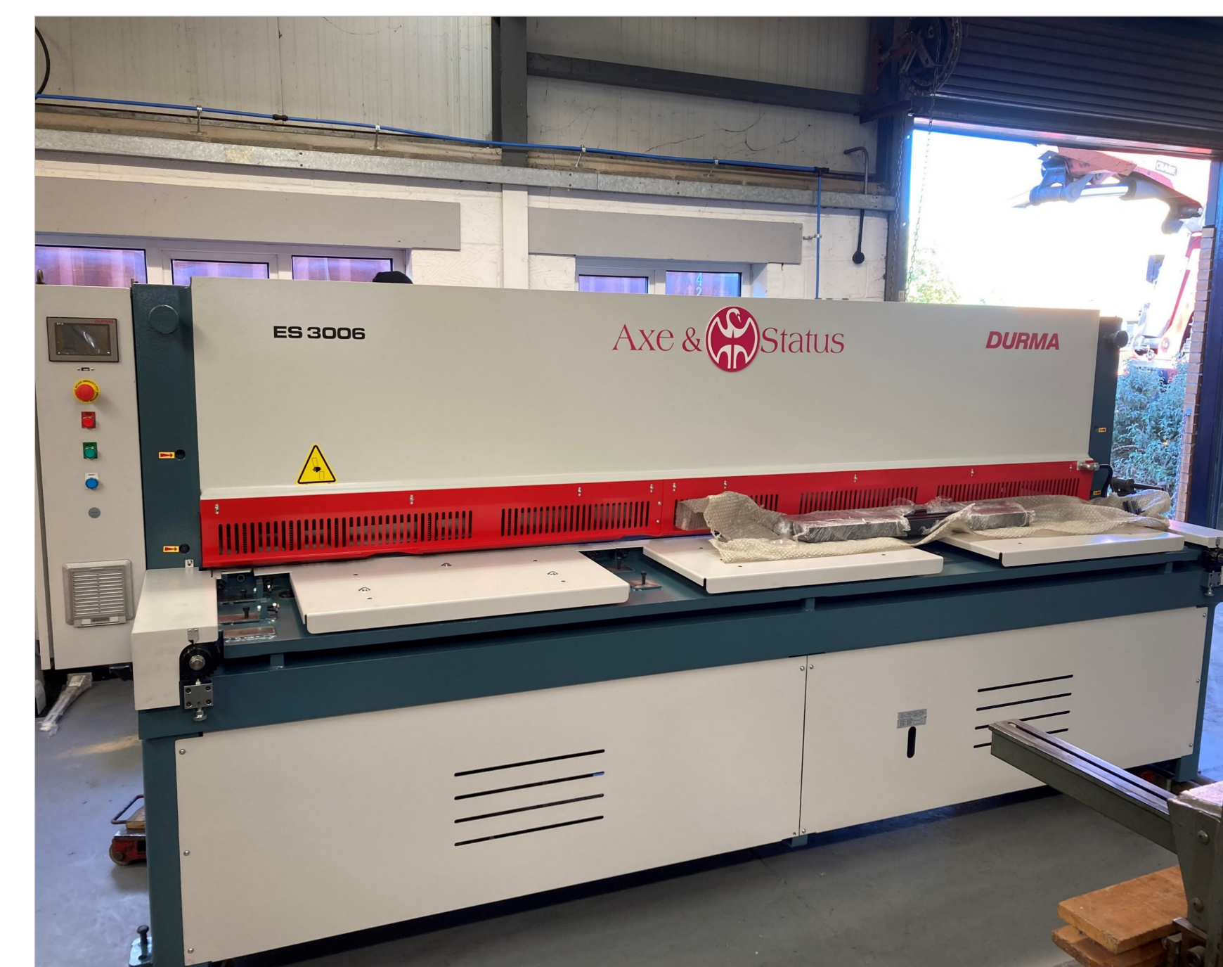
3 m NC controlled guillotine
